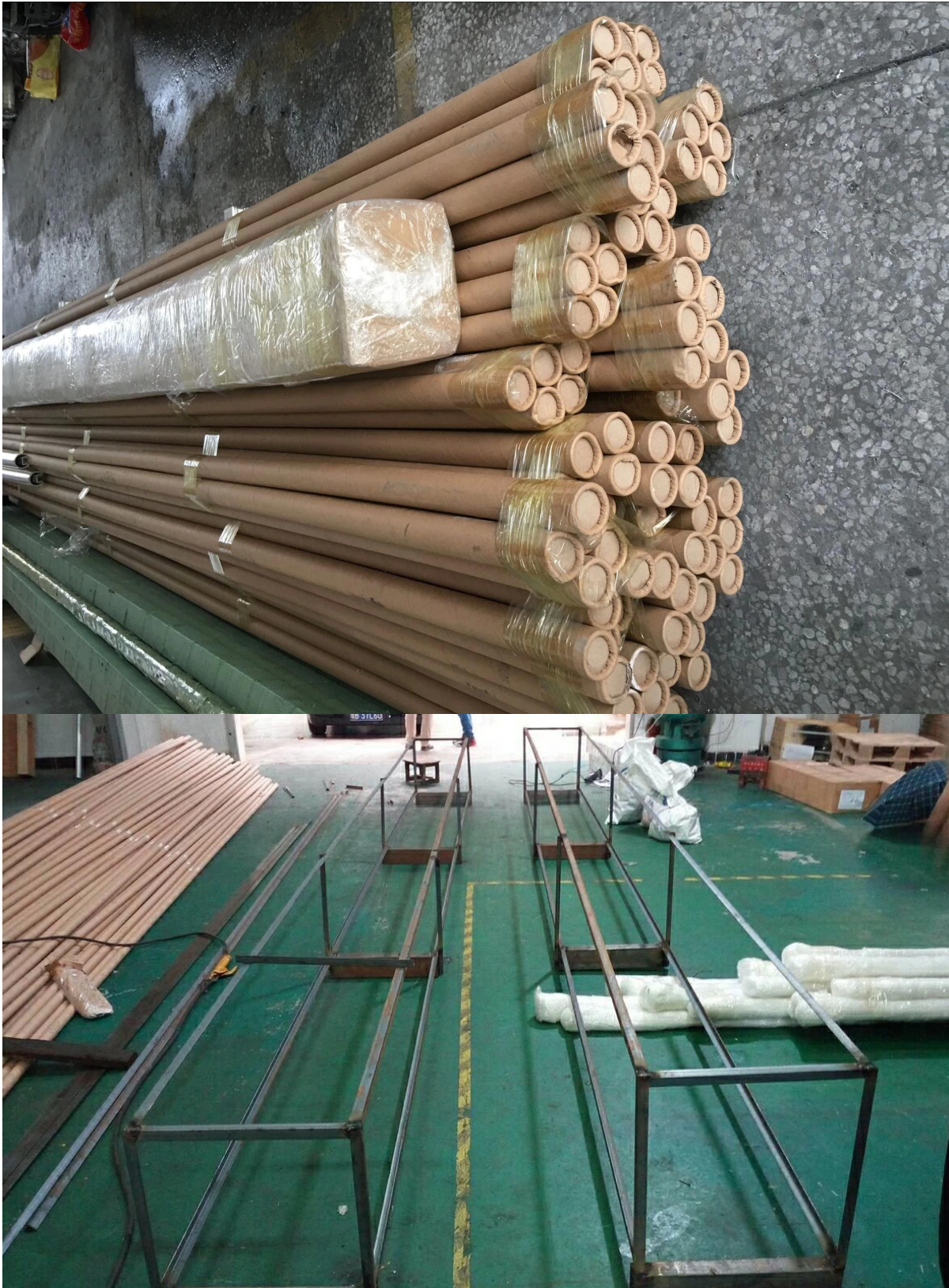
Installation photos of 20x25mm stainless steel 316L slot tubing for 12mm glass
