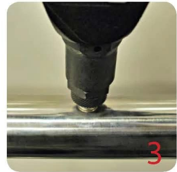
Insert blind rivet nut into tube and fasten with blind rivet tool.
