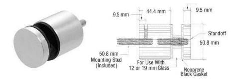
We actually production drawing, as customer request, which fitting for 12mm glass:
