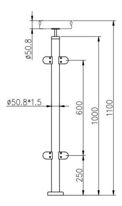
3. Hand rail 90 degree corner post **LCH-108** (135 degree and customer degree available)
