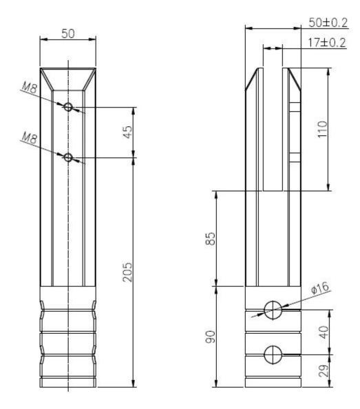
This model of spigot can be used for pool fence and balcony fence. It's much stronger than base mount spigot. Its heavier and size bigger than base mount models. Each spigot is about 1.9KG.
