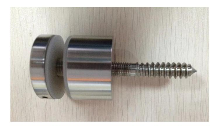
model No.: SF-50 material: stainless steel 304/316 finish: satin /mirror polished size: 50\*10mm cap,50\*30mm body, M12\*120 bolt, silicon rubber gasket included to fit 10-19mm glass
