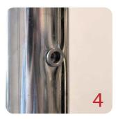
Check installed blind rivet nut is secure and ready for install.
