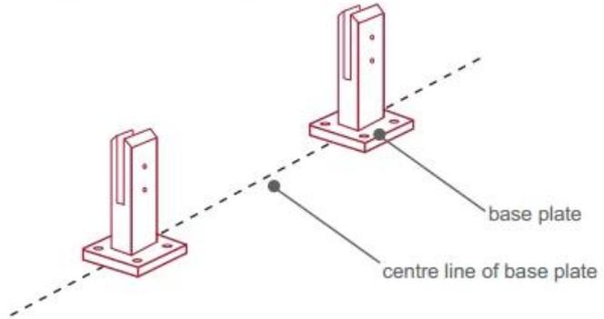
Now the base plated spigots can be fitted to the floor and plumbed via shims (not supplied) under the base plates. Be sure to tighten firmly as the smallest of movement at the base plate will result in noticeable movement at the bottom of the glass fence.
