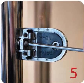
Align half glass clamp with blind rivet nut inline position. Screw in button head cap screw into thread and tighten with hex key.
