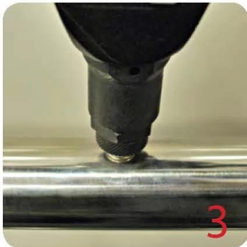
Insert blind rivet nut into tube and fasten with blind rivet tool.
