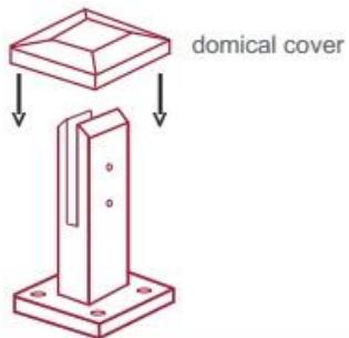
The glass is then installed to the spigots.
