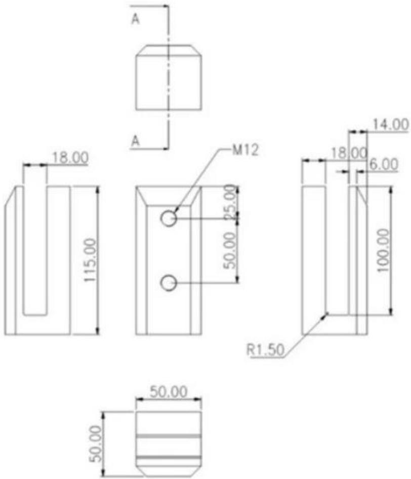
1. Suit for M12\*120mm machined bolt for concrete
