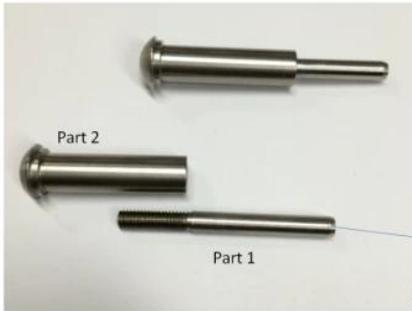
Put cable inside part 1 and tighten with hydraulic crimper , then let part 2 go Through post and then screw together With part 1 .
