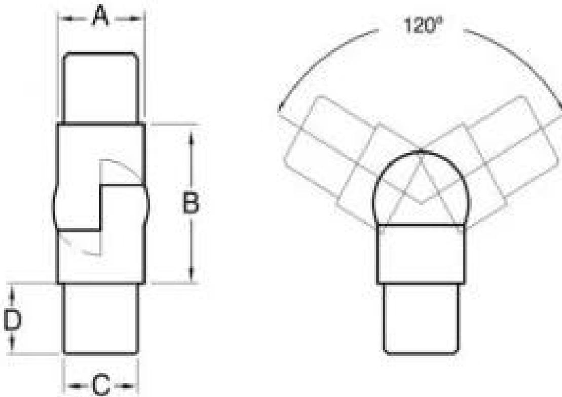
**Description:** The joint to connect 20mm tubes with graduations between 90° and 180°.
