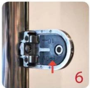
Select appropriate rubber gasket to suit glass panel thickness. Install rubber gasket into both sides of glass clamp. (Note rubber gasket marked with sizes).
