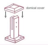
The glass is then installed to the spigots. Place plastic packers between glass & spigot, at no stage should glass touch the metal How adjustability works:
