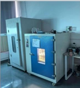
. Aging Test device
