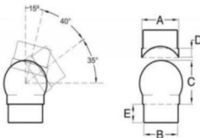
**Description:** Spherical joint to connect handrail with graduations between 90° and 180°
