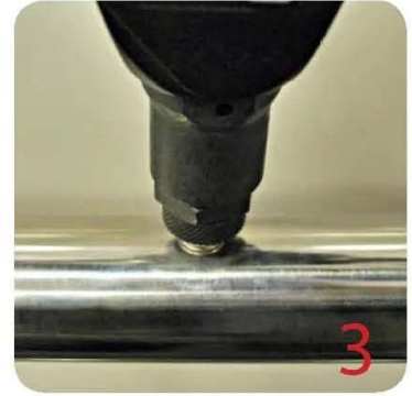
3 Insert blind rivet nut into tube and fasten with blind rivet tool.
