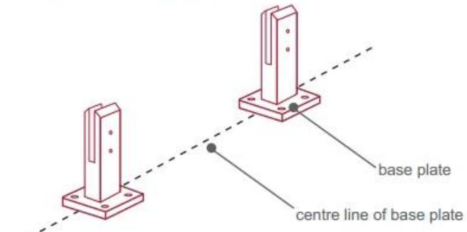
Now the base plated spigots can be fitted to the floor and plumbed via shims (not supplied) under the base plates. Be sure to tighten firmly as the smallest of movement at the base plate will result in noticeable movement at the bottom of the glass fence.
