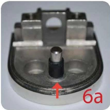
6a If heavier clamping load is required please use supplied glass clamp pin, during the install process. Note glass panels will require drilling in order to fit glass clamp pins.
