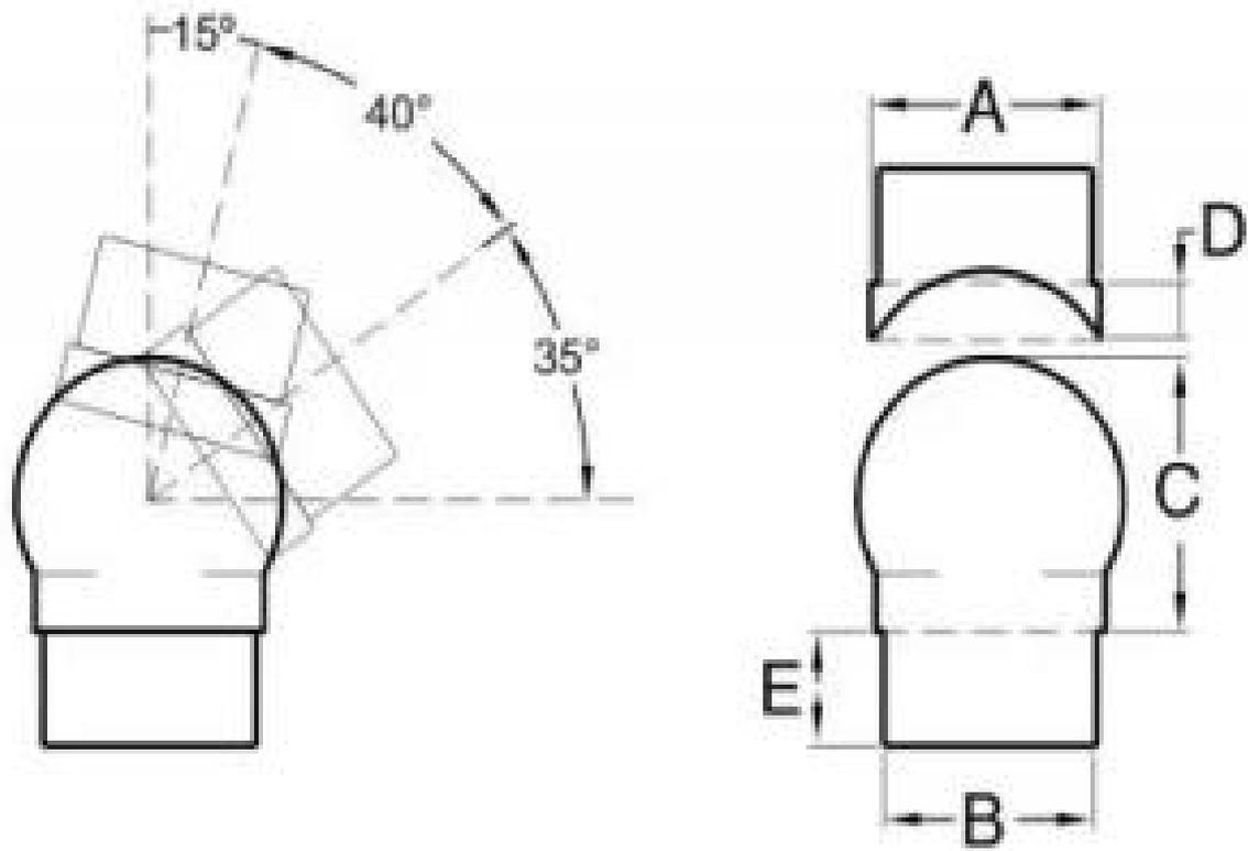
**Description:** Spherical joint to connect handrail with graduations between 90° and 180°
