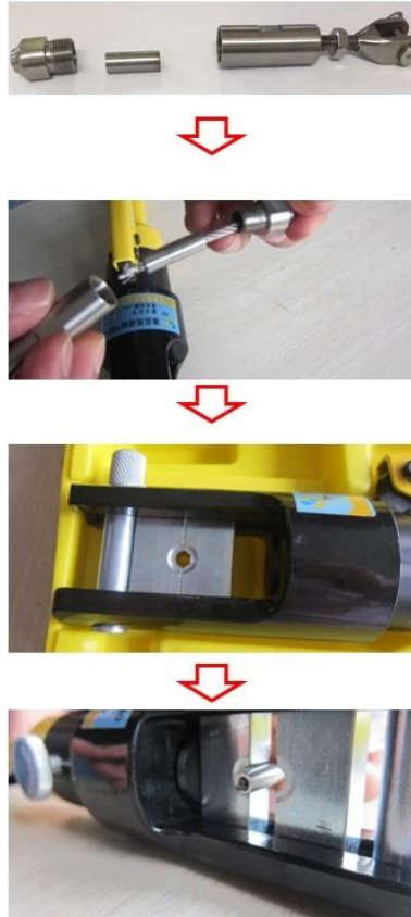
Type 2: with hydraulic crimper
