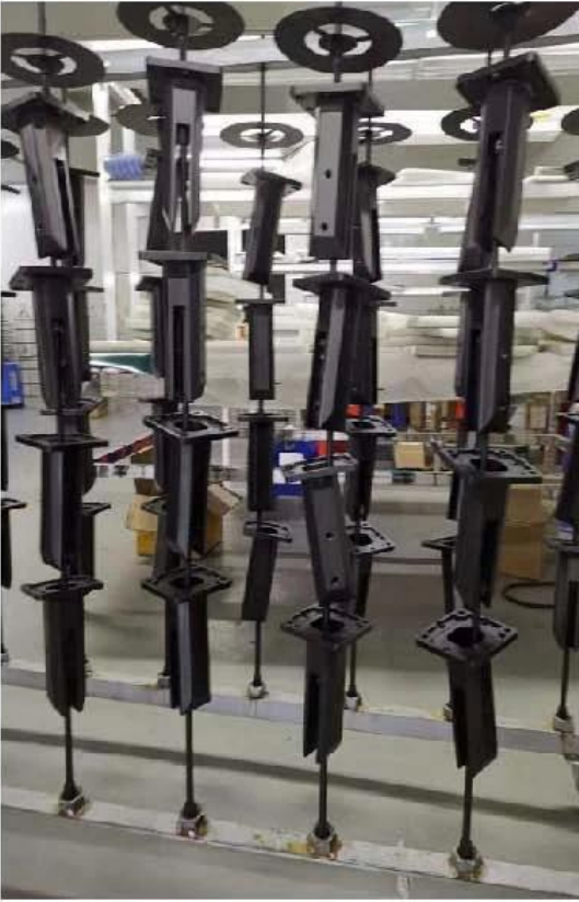
MATT BLACK ELECTRO PLATING PROCESS
