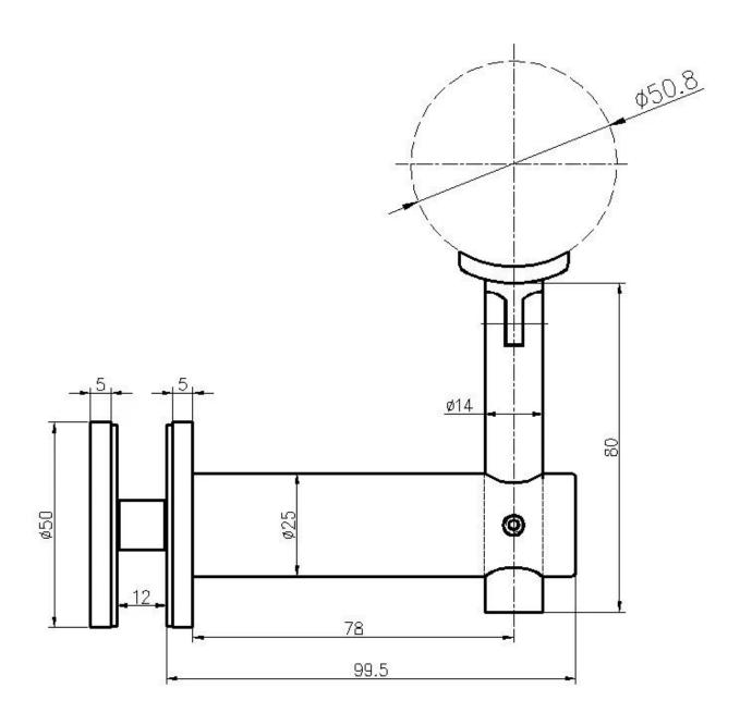
**#Production photos of Adjustable Glass-mounted handrail bracket -**
