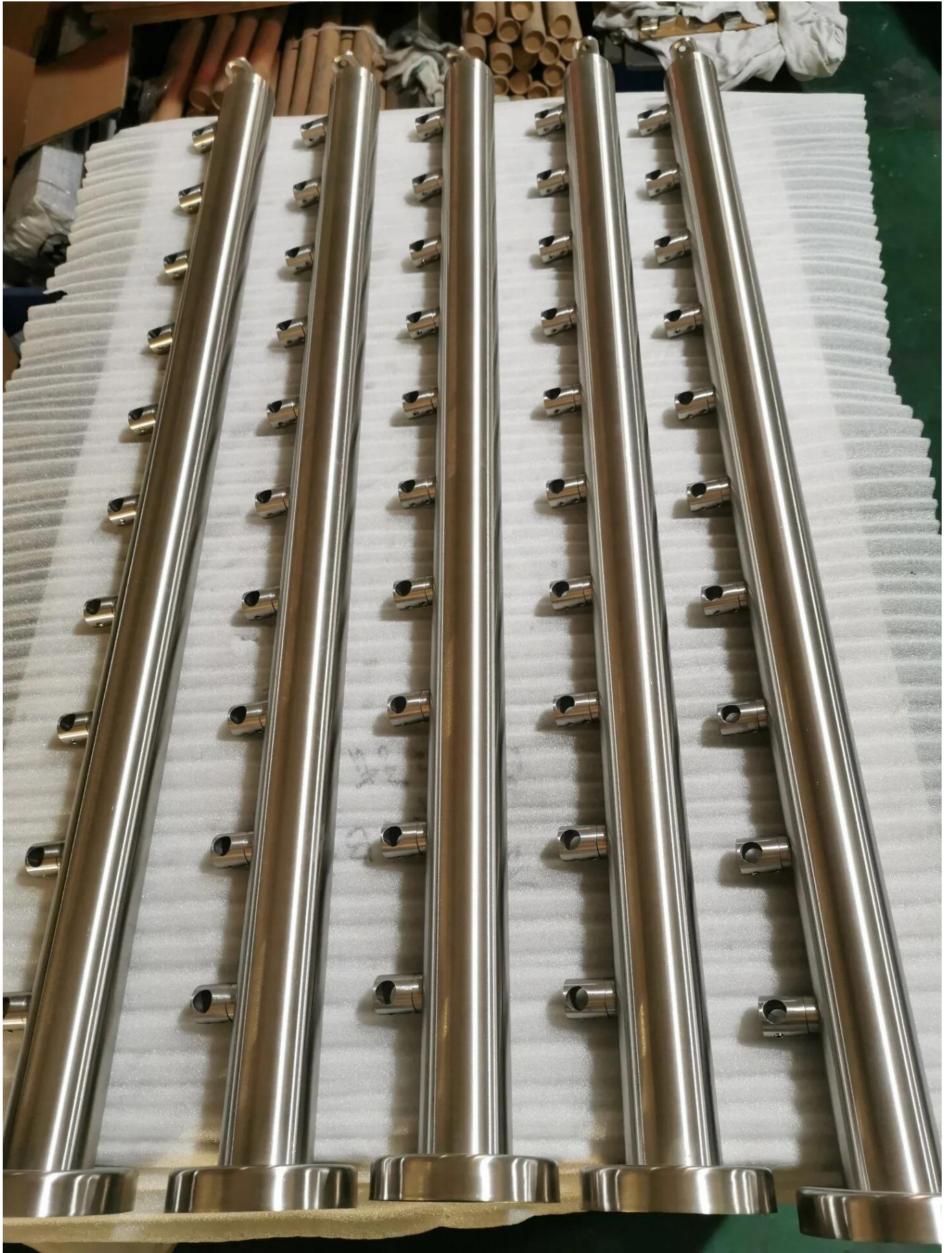
Production photos of stainless steel crossbar balustrade post
