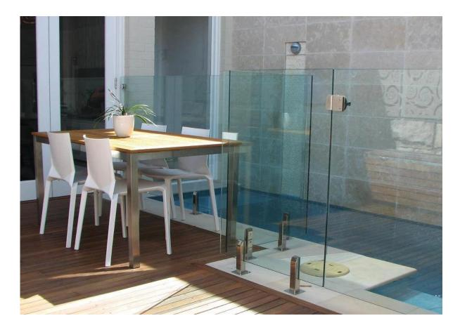
\* indoor glass railing with slotted handrail (with SBM spigot)
