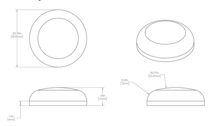
Other designs of handrail fitting stainless steel pipe end caps:
