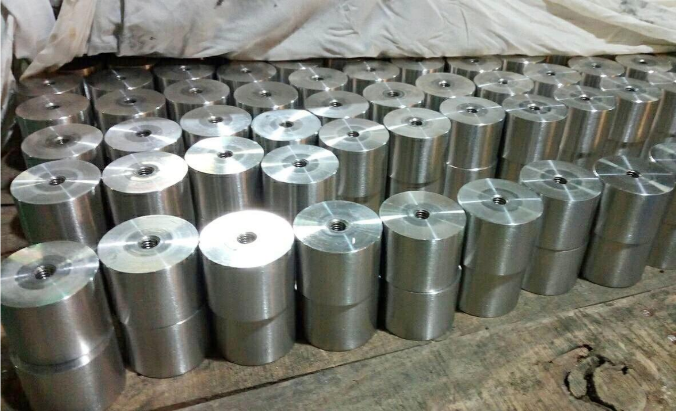
2" stainless steel standoff in frameless glass staircase railing project :
