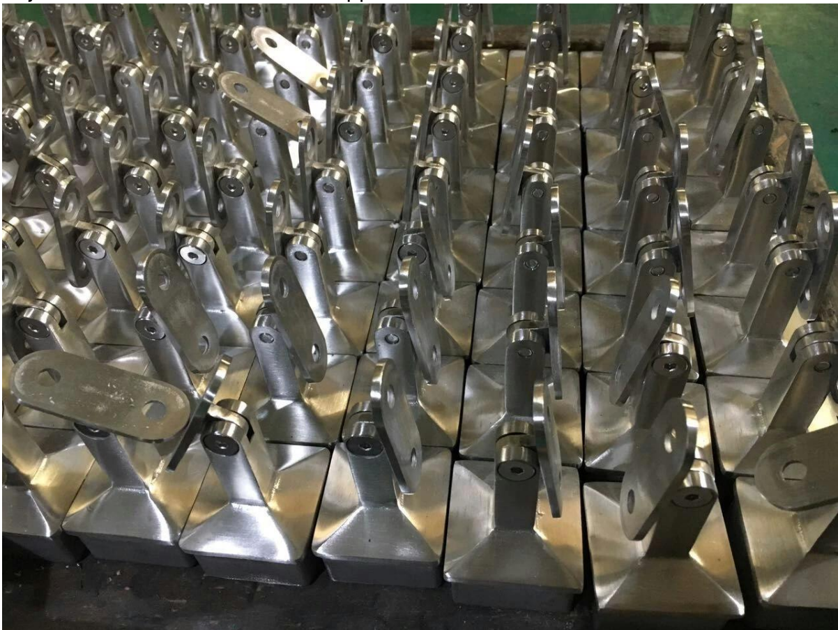
Fascia mounted square post for cable railing
