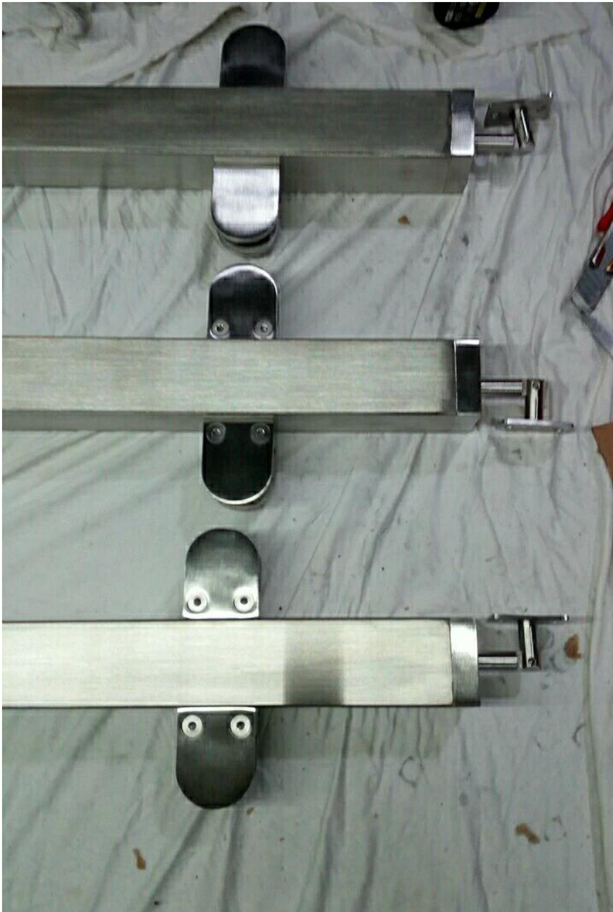
Fascia mounting/side mounting balustrade handrail post Weld a plate on side first, then attached with 2 screws
