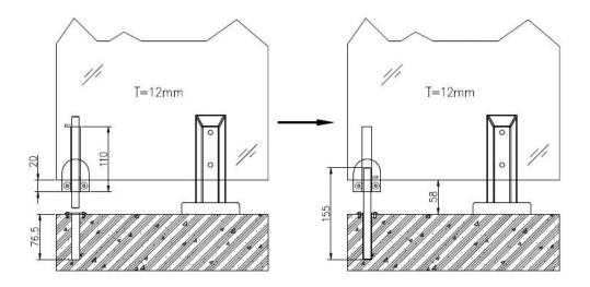
Glass door stopper is used at the bottom of glass door, to keep it opening or closing; The installation is very easy and fast, just like the glass clamp.
