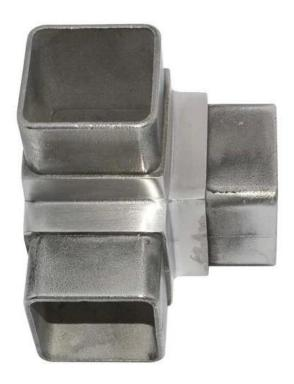
Tube connector **\$404**Connects to 40x40mm, 1.3-1.5mm thick tube
