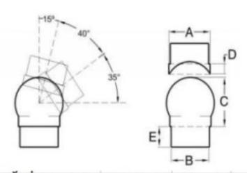
Description: Spherical joint to connect handrail with graduations between 90° and 180° 描述,球面接头连接楼梯扶手从90°到 180°范围变化。
