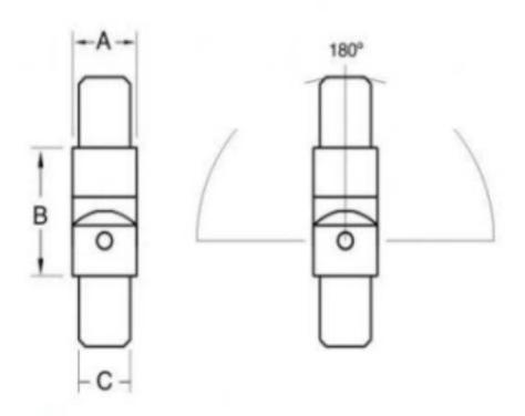
Description: The joint to connect 12mm tubes with graduations between 90° and 180°.
