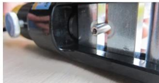
T804 , swage type , need hydraulic crimper -
