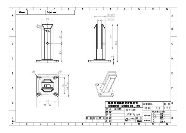
Round type surface mount friction fit glass spigot  $\mbox{RBM-2}$  Net weight:1.32kg/piece Hight: 168mm Base plate size:  $\phi100\mbox{mm}$
