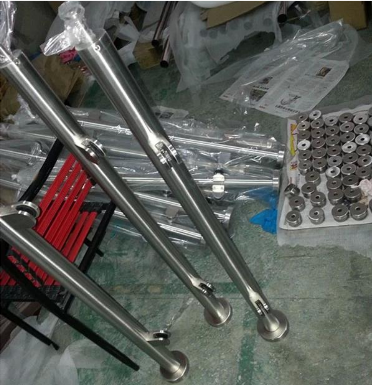
End cap required stainless steel balustrade post
