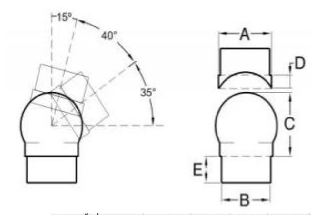
Description: Spherical joint to connect handrail with graduations between 90° and 180° 描述: 球面接头连接楼梯扶手从90° 到 180°范围变化.
