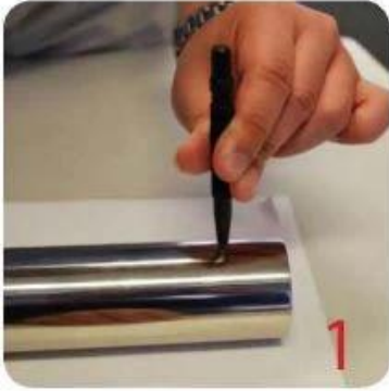
Mark and centre punch desired location of blind rivet nut location.
