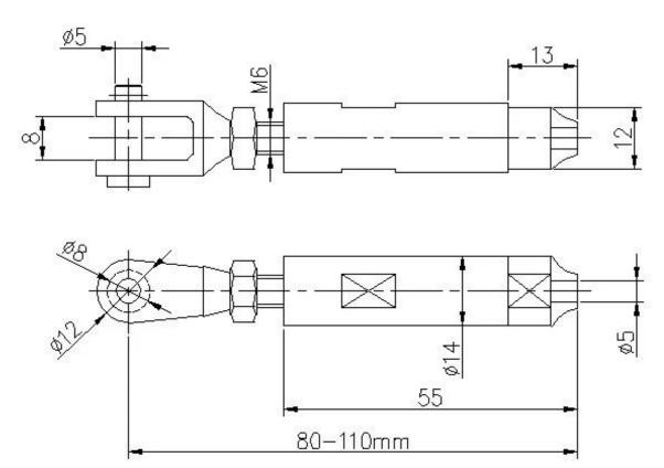
$\underline{\text{Inside structure of T803 cable tensioner , clip tight type , no need hydraulic crimpers -}\\$
