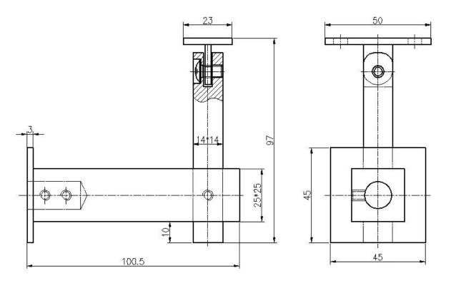
Project photos of wall mount square handrail support bracket for square tubing handrail:
