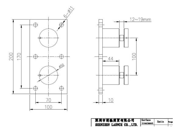
SF-50T is used for big size and heavy glass such as 12mm, 15mm, 19mm or more. It could be used at balcony, deck, staircase at indoor or outdoor.
