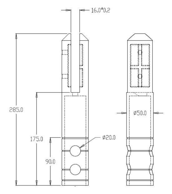
This model of spigot can be used for pool fence and balcony fence. It's much stronger than base mount spigot. Its heavier and size bigger than base mount models.
