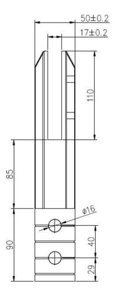
This model of spigot can be used for pool fence and balcony fence. It's much stronger than base mount spigot. Its heavier and size bigger than base mount models.
