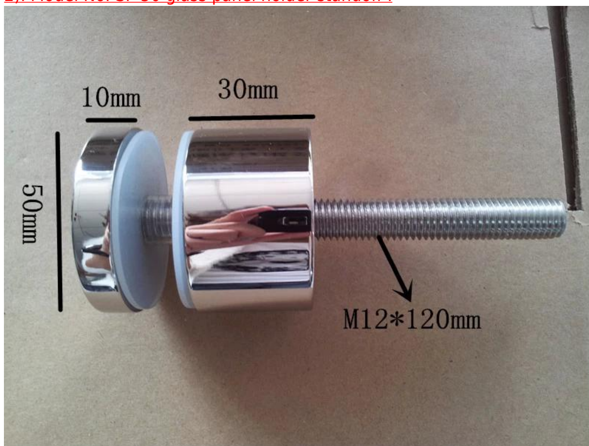
2). Model No. SF-50 glass panel holder standoff.
