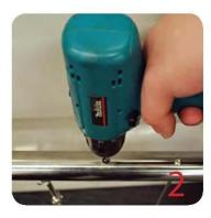
Drill centre punched hole in tube to suit blind rivet nut.
