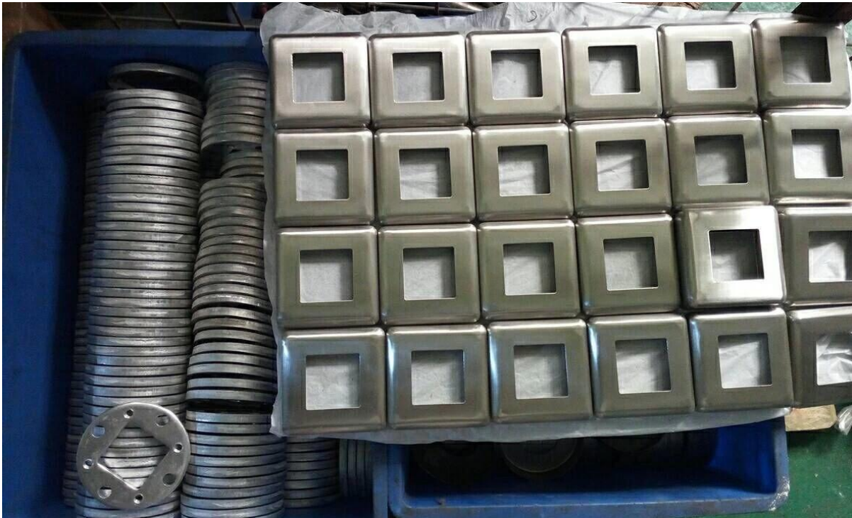
Base plate for posts ( will be welded to post at our factory)
