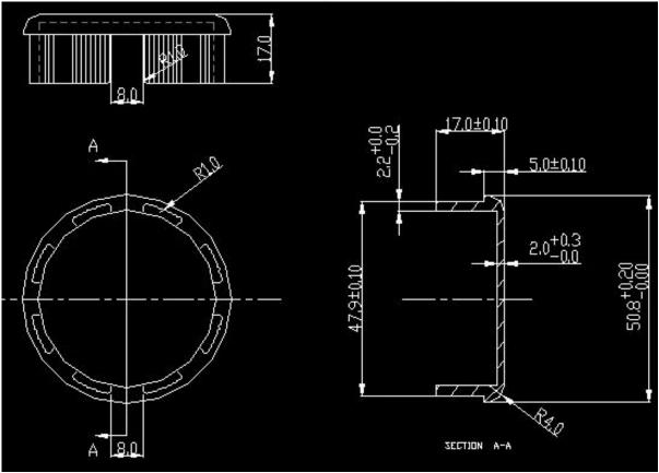
3. Photos of stainless steel push fit end cap for 2 inch tubing
