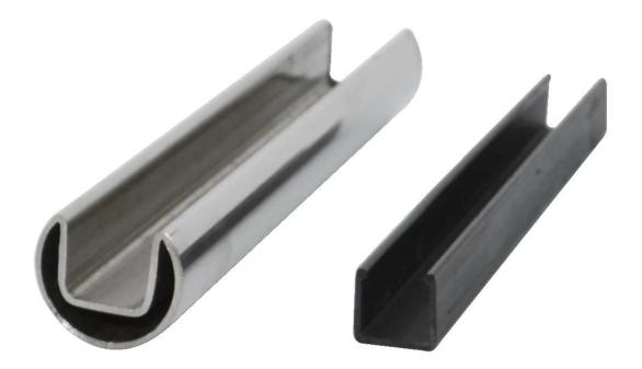
material: stainless steel 316 finish: satin or mirror polished dimension: dia 25.4mm, groove 14\*14mm, 5.8 meter per length fittings: round 180 degree connector, 90 degree connector, wall to rail connector, end cap for glass thickness: 12mm
