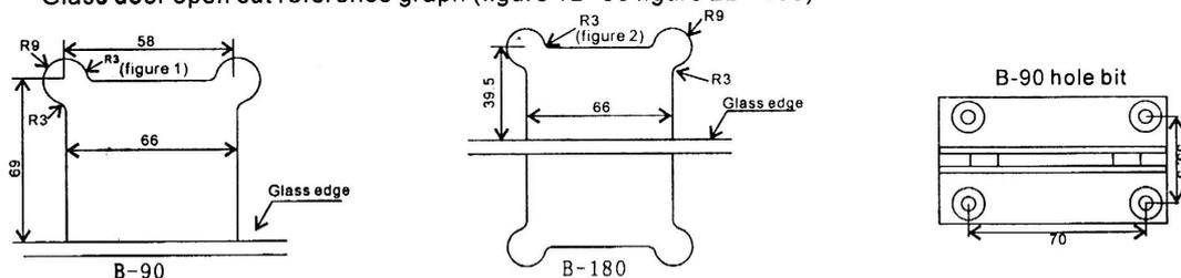
After the glass cut , it must be treated with steel processing ,make sure the installation angle between the glass door and the ground is 90°when you install it .
