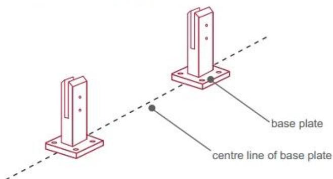
Now the base plated spigots can be fitted to the floor and plumbed via shims (not supplied) under the base plates. Be sure to tighten firmly as the smallest of movement at the base plate will result in noticeable movement at the bottom of the glass fence.
